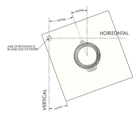
The sensor measures the angle ALPHA about the axis of rotation as shown above. It is not a requirement that the sensor be mounted on the axis of rotation.
